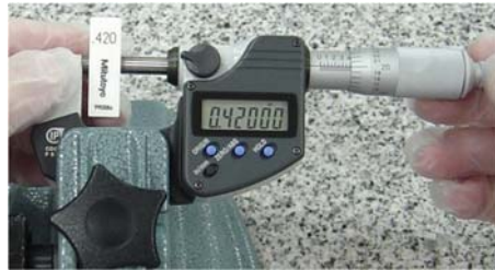
Micrometer calibration using a gage block.
