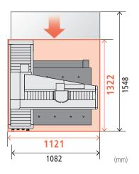
The storage cabinet for PC, machine controllers, etc., under the measuring table reduces the footprint by about 20 % when compared with that of other coordinate measuring machines with similar measuring range.
