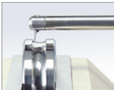
Inner/outer ring contour of a bearing
