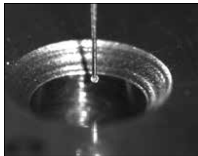
MPP-NANO micro-hole measurement
