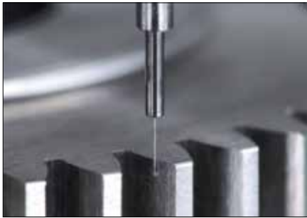
Module 0.8 master gear measurement
